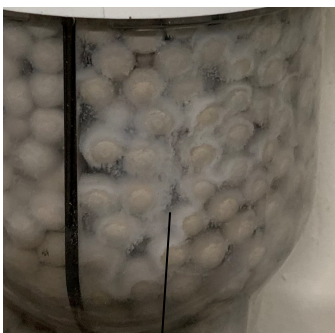
Figure 4: Salt precipitate deposited on neutralization media from Aluminum heat exchangers
