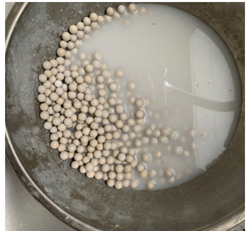
Figure 4: Neutralization media that has been rinsed with clean water
