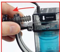
1. Loosen the thumb screw
