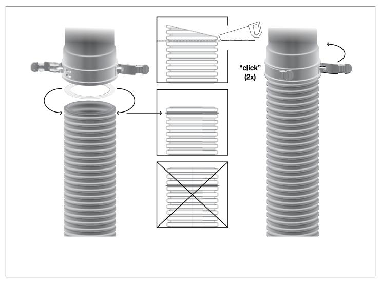
Mount the seal into the first whole groove from the cut end and push the flexible liner into the adaptor until it stops. Hold the adaptor to the liner with the latching tabs. It is possible to loosen the latching tabs with a screw driver.
