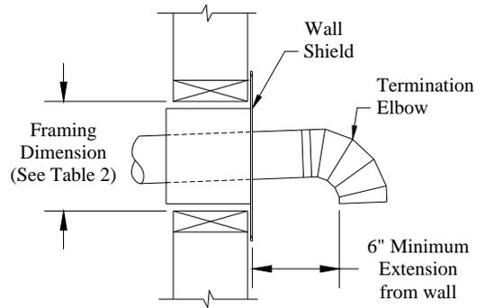
**Fig 16. (Wall Shield & Termination Elbow)**
