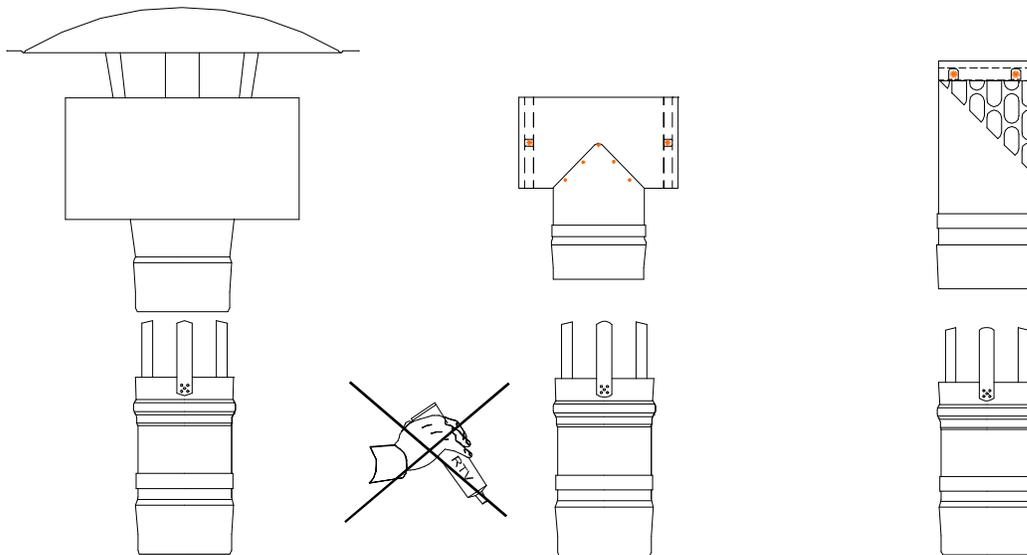
**Termination attaching to EZ Seal, NO sealant required.**
