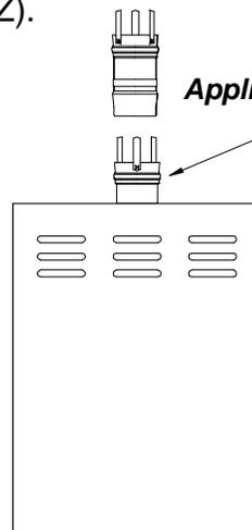
***Appliance flue collar has Heat-fab's integral red seal.
