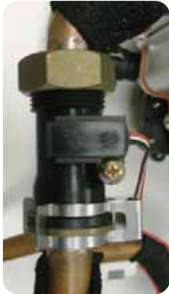
1. Drain water, and unfasten the upper nut of the flow sensor.
