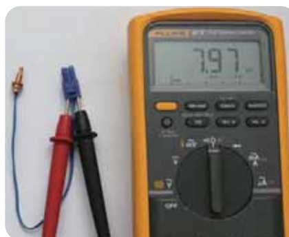
< Check if the hot water temperature sensor is open >
