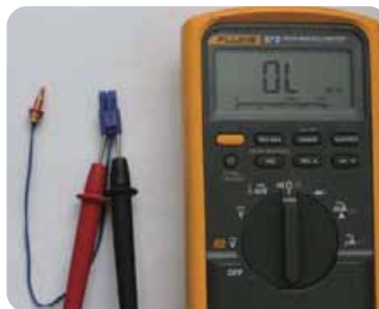
<Check if the hot water temperature sensor is open> Error type : MΩ Open
