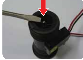
4. If the impeller does not rotate, disassemble it by pushing the axis with a driver.
