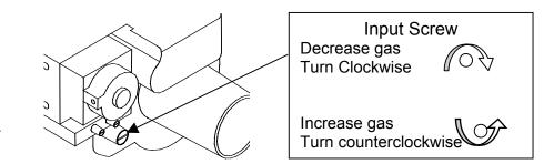
IF FOR ANY REASON THE INPUT SCREW IS ADJUSTED, A "COMBUSTION ANALYZER" MUST BE USED TO ENSURE SAFE AND PROPER OPERATION.
