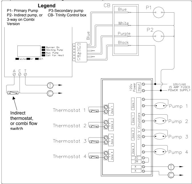
The basic multiple zoned system using circulating pumps. This wiring system is used with the piping as described in 6.2.2 Multiple Zones using Pumps and 6.2.3 Multiple Zones with different temperatures.
