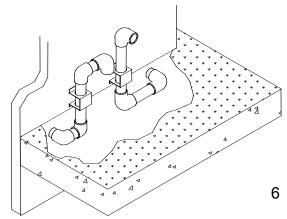
Excavate site as shown in figure, to a point below where the pipes are to exit. Ensure that the wall is fully sealed where the pipes penetrate the wall. The vent piping MUST be secured to the side of the building above grade, as shown, to provide rigidity. NTI Provides a mounting bracket PN. 82075 for securing the exhaust pipes. Ensure that the vent clearances are maintained (Inlet minimum 12" plus snow allowance from grade, exhaust outlet 18" minimum above inlet).
