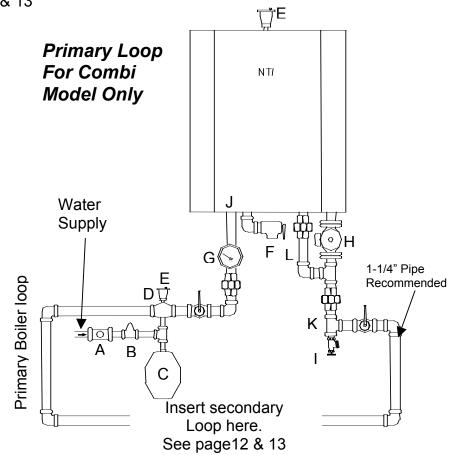
**Flow:** The Trinity boiler must have water flow going through the boiler whenever the burner is on.
