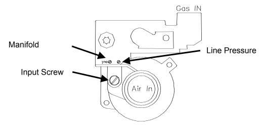
The input Screw "MUST NEVER BE ADJUSTED" unless you have a calibrated combustion analyzer to verify the combustion properties are within normal operating ranges.
