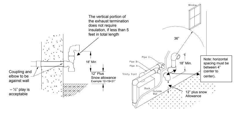
Concentric vent terminal Use NTI part # 82666 or York Part# 1CT0303 Clearances and requirements of this manual supersede, those of the Instructions enclosed in vent terminal #650.75-N2, which contain more detailed assembly instructions.
