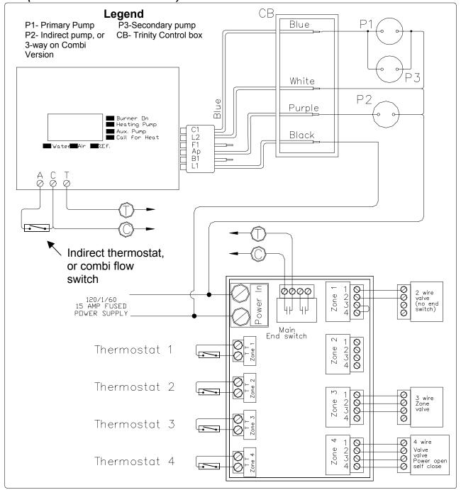
The basic multiple zoned system using normally closed 2 – 3- or 4 wire Taco zone valves. This wiring system is used with the piping as described in Section 6.2.1 "Multiple Zones using Zone Valves".
