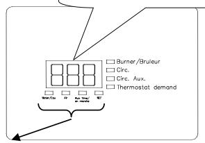
Water/Eau = When illuminated, indicates that the display is showing boiler water temperature.
