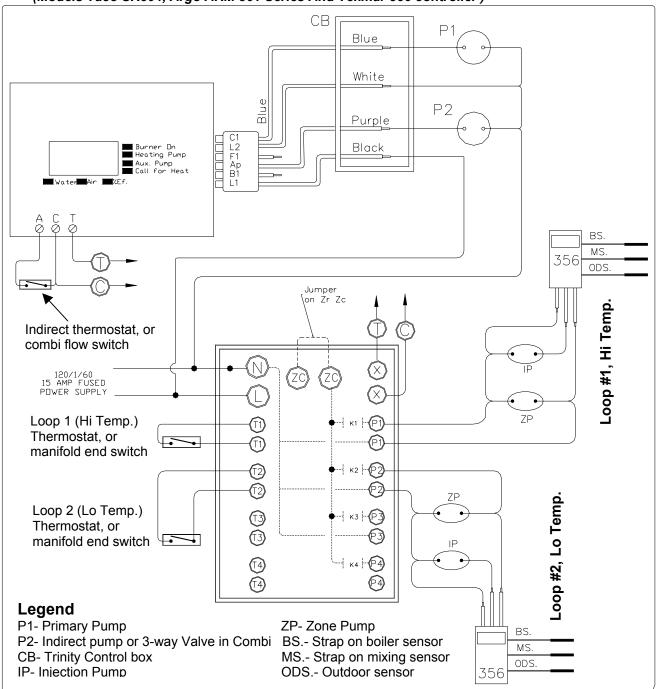
This wiring system is used with the piping as described in 6.2.3 Multiple Zones with different temperatures ((Using Injection pumps))
