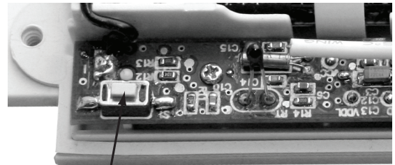
Connection button located inside the RZ250W
