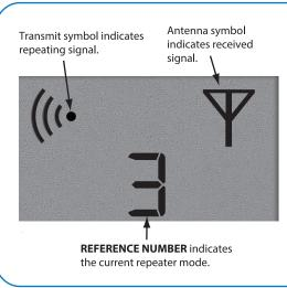
When the W150W receives a wireless signal to repeat, the **PRecieved Symbol** will flash. After a few seconds the Red Indicator Light ① and the ((• **Transmit Symbol** will flash. Indicating a repeated signal.
