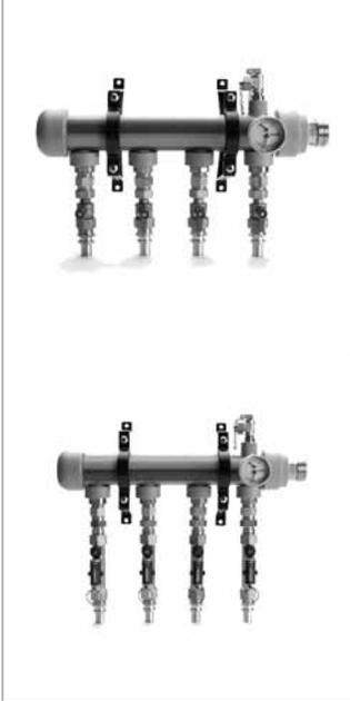
REHAU's robust PRO-BALANCE XP Manifold for larger flow capacity applications is constructed from a strong, durable polypropylene material and is available in 4 to 20 drops. The XP manifold can connect to either 1 or 1 1/4 in. RAUGEO PEXa pipe using REHAU's EVERLOC fittings. Manifold pipe diameter varies according to number of drops. 2 or 3 in. MPT connection to main. See product submittal for details.
