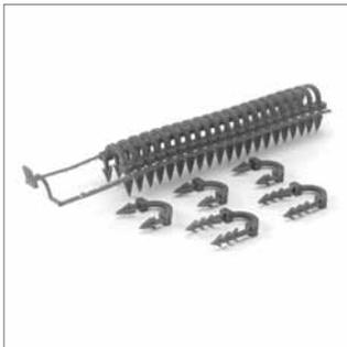
RAUTACK 3D 1 3/8 in. staples work with 3/8, 1/2 and 5/8 in. pipe. RAUTACK 3D 2 3/8 in. staples are required for 3/4 in. pipe, but also work with 3/8, 1/2 and 5/8 in. pipe. Typically, one staple is required every 3 ft (90 cm) on straight runs of pipe with an additional staple in the middle of bends. RAUTACK 3D staples are installed from a standing position using the RAUTACKER 3D stapler tool. Follow all published installation instructions.
