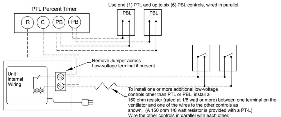
\* Except when ERV is operating due to an additional control wired directly to the unit.
