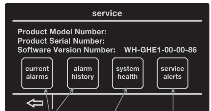
Current Alarms and Alarm History allows you to access any current alarms that have been tripped and view a list of previous alarms.
