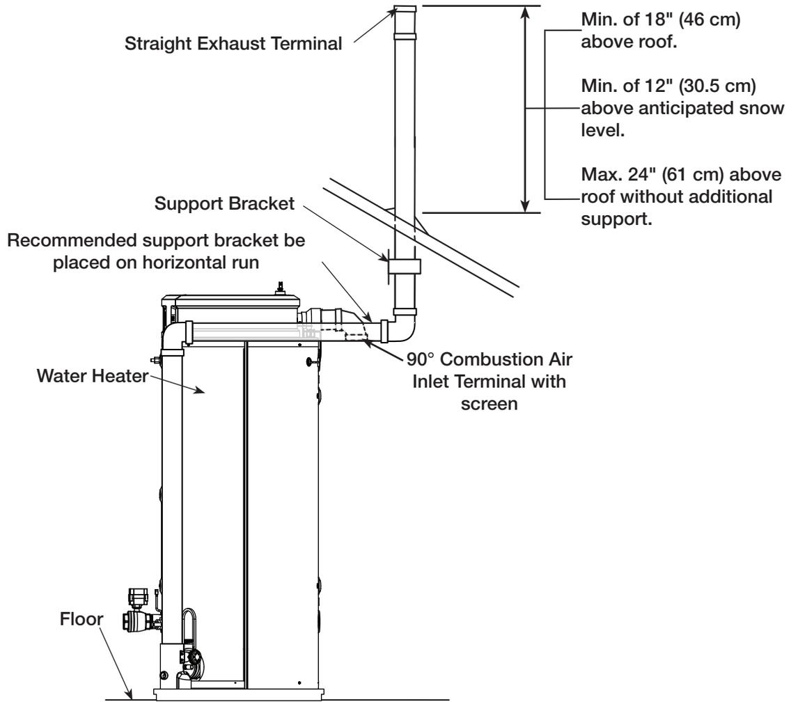
Alternate vertical venting with exhaust vent turned down - preferred for cold climates.
