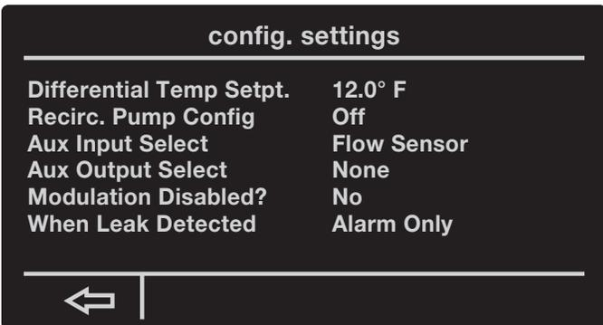
The setting can be highlighted by tapping and then adjusted with the up/down arrows.
