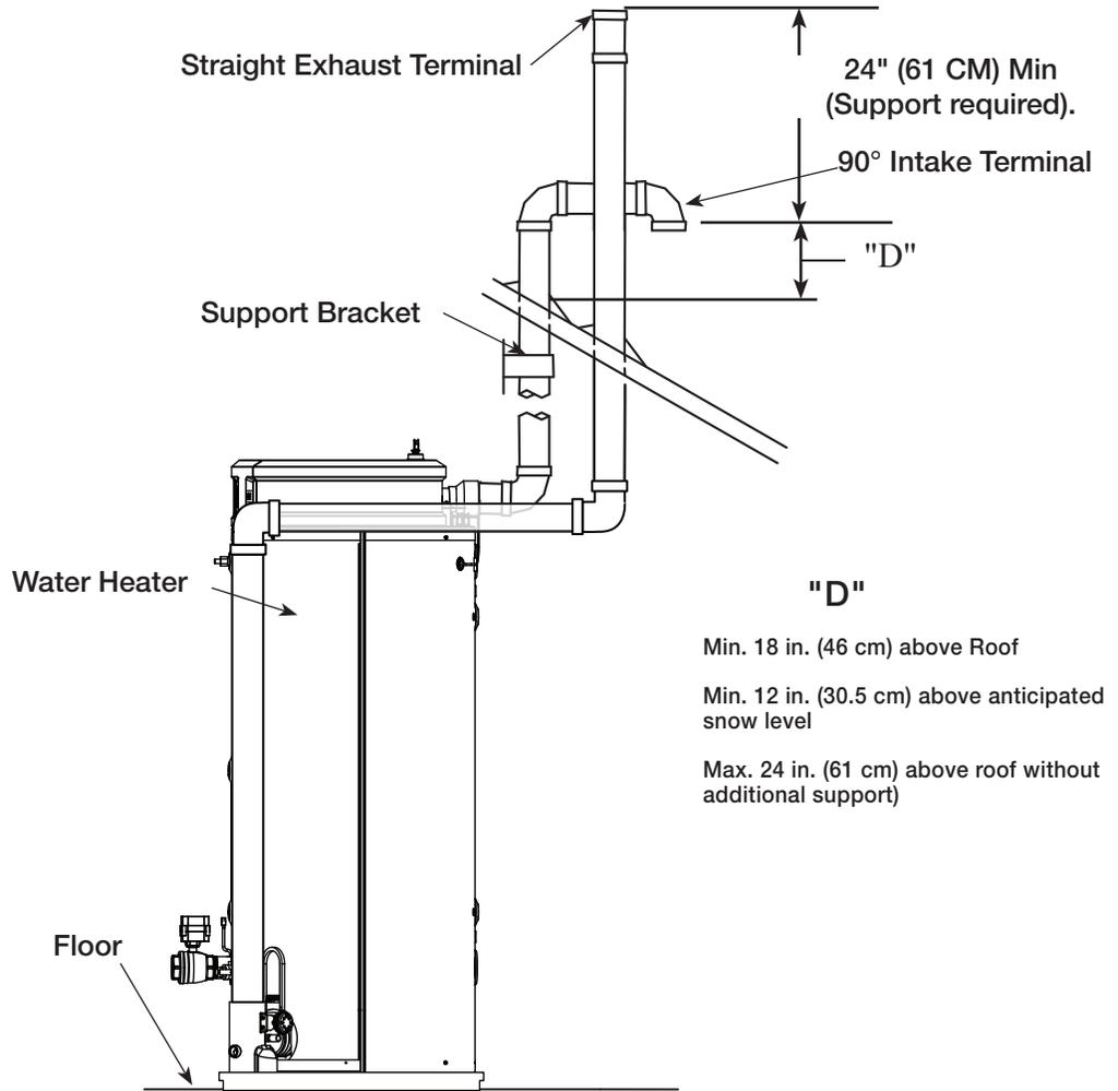
Alternate vertical venting with exhaust vent turned down - preferred for cold climates.
