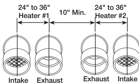
Figure 12b: Multiple Unit Venting
