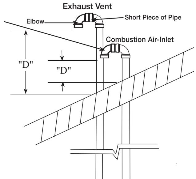
Terminals spacing for horizontal or vertical venting.
