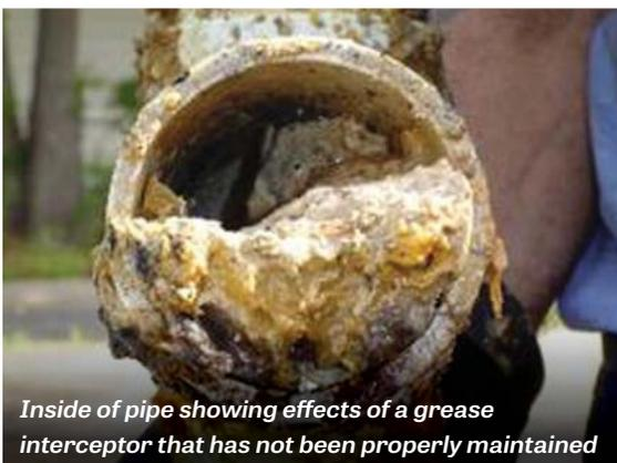
*Inside of pipe showing effects of a grease interceptor that has not been properly maintained*
