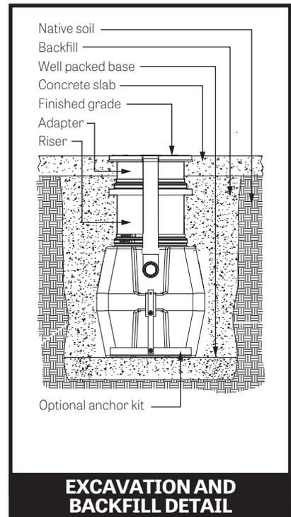
**EXCAVATION AND BACKFILL DETAIL**
