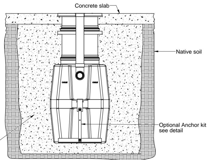
**EXCAVATION AND BACKFILL DETAIL
