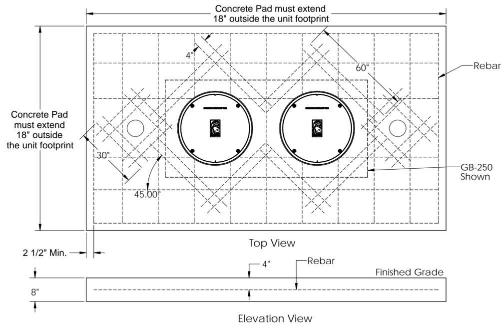
**CONCRETE SLAB DETAIL FOR TRAFFIC LOADING
