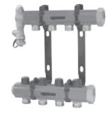
The TruFLOW Jr. Assembly with Balancing Valves and Valveless manifold comes fully assembled and ready for installation. The manifold body ends have R32 unions and the loop outlets have QS20 male threads.
