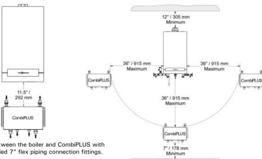
Min. distance between the boiler and CombiPLUS with Viessmann supplied 7" flex piping connection fittings.
