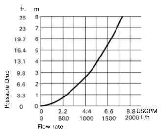
A low-loss header **must** be used when the **system** flow rate exceeds the maximum (or minimum) flow rate of the Vitodens 100-W boiler. An alternative method may be used, such as primary secondary piping using closely spaced tees.
