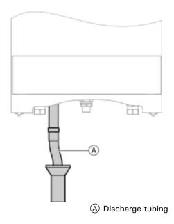
The condensate drain of the Vitodens 100-W boiler is equipped with a built-in siphon trap in order to keep flue gases from being discharged via the condensate drain.
