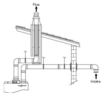
Flexible two pipe system (room air independent)
