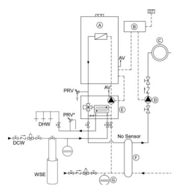
Note: The use of a low-loss header is recommended if the water flow rate is less than 1.7 GPM (400 L/h) or more than 6.2 GPM (1400 L/h).
