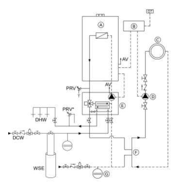
Note: The use of a low-loss header is recommended if the water flow rate is less than 1.7 GPM (400 L/h) or more than 6.2 GPM (1400 L/h).
