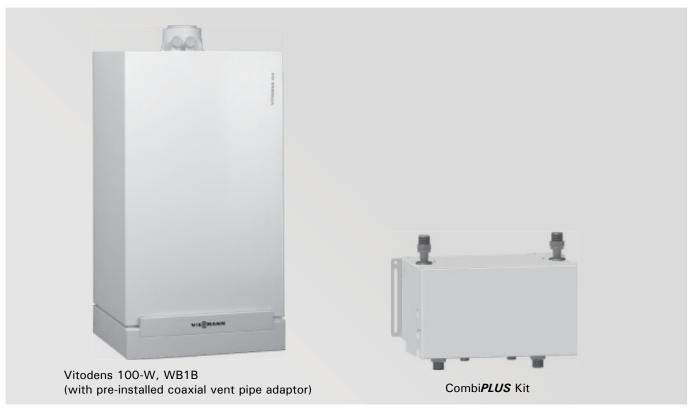
Gas-Fired Wall-Mounted Condensing Boiler with modulating stainless steel MatriX cylinder burner, stainless steel Inox-Radial heat exchanger for room air independent operation (using a direct vent system) or room air dependent operation. Optional CombiPLUS Kit providing reliable on demand hot water without a DHW tank is available.
